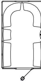
Sedna Model 8 Steam Room Size: O.D. 2330mm x 3853mm Height: O.D. 2265mm 11 Person seating capacity. 11.4kW - 1 or 3 Phase
